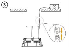
Align pins and connect wires together. Twist locking sleeve until secure.
