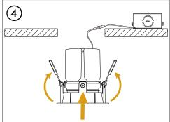
Push spring clips up and insert into ceiling cutout.
