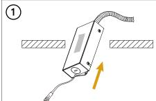
Insert driver through ceiling cutout, leaving access to quick connect wire. Secure the driver with double sided tape.
